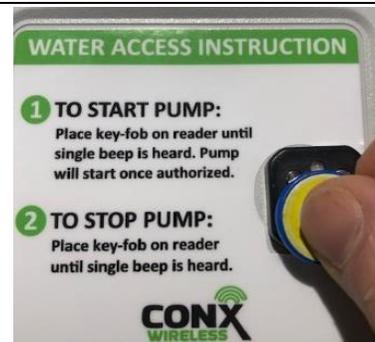
**Step 2 – Await Authorization, Pump Turn On:** Once authorized, the pump will start automatically (two beeps will signal authorization; fob reader will illuminate red).
